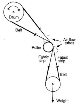
FIGURE 1. Arrangement of TRI fabric/fabric abrader.
