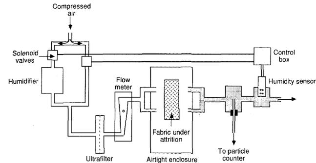
FIGURE 2. Apparatus for collection and sampling of airborne particles generated during fabric abrasion.
